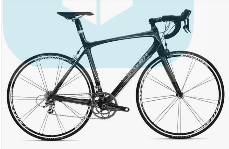
Figure 3-5: The short wheelbase of a road bike makes it responsive to turns, and its frame geometry allows you to feel more comfortable on extended rides.
